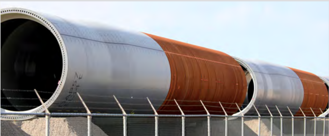
Figure 1. Large mono piles with circumferential welds
