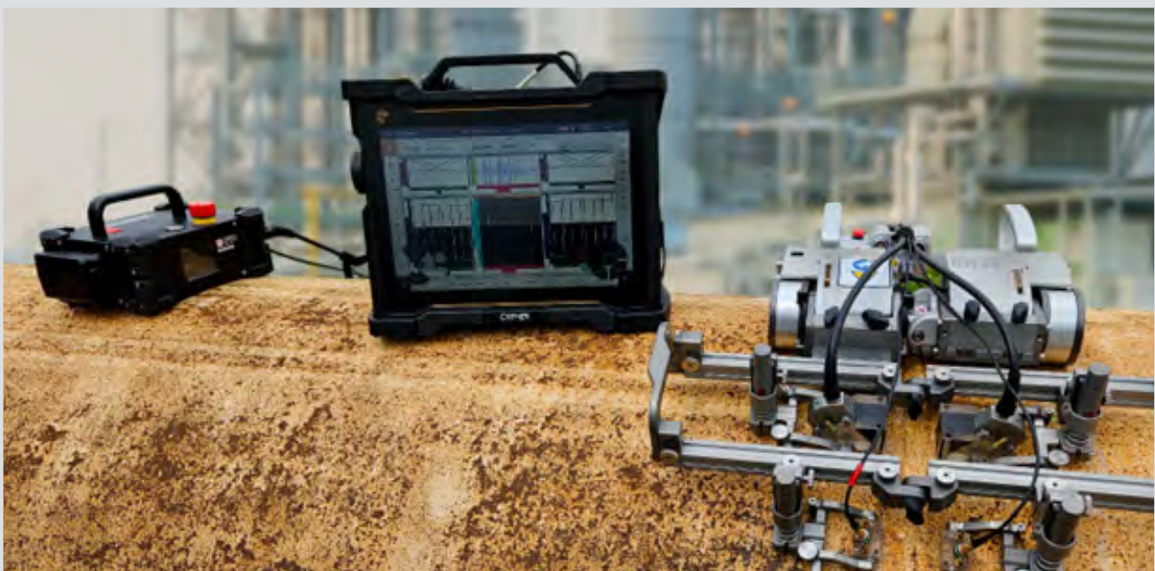
Figure 3. Cypher® automated weld inspection system with PWI and TOFD using a Jireh Navic weldscanner
